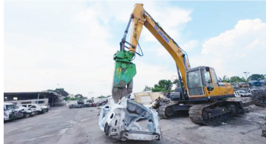
An excavator fitted with a hydraulic shear attachment dismantles an end-of-life vehicle at Standard Insurance’s ELV (End-of-Life Vehicle) dismantling facility
